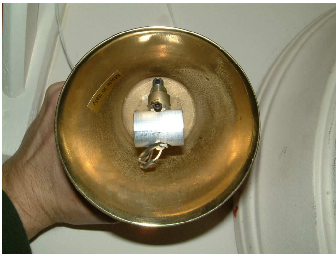
A 24VDC Solenoid mounted inside of a 4" Bell for Hour Strike
